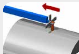
Outside or inside welding of a longitudinal seam
