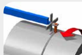
Outside or inside welding of a circumferential seam
