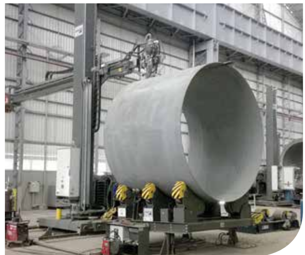
Longitudinal PEMA welding station with HD series Column & Boom.
