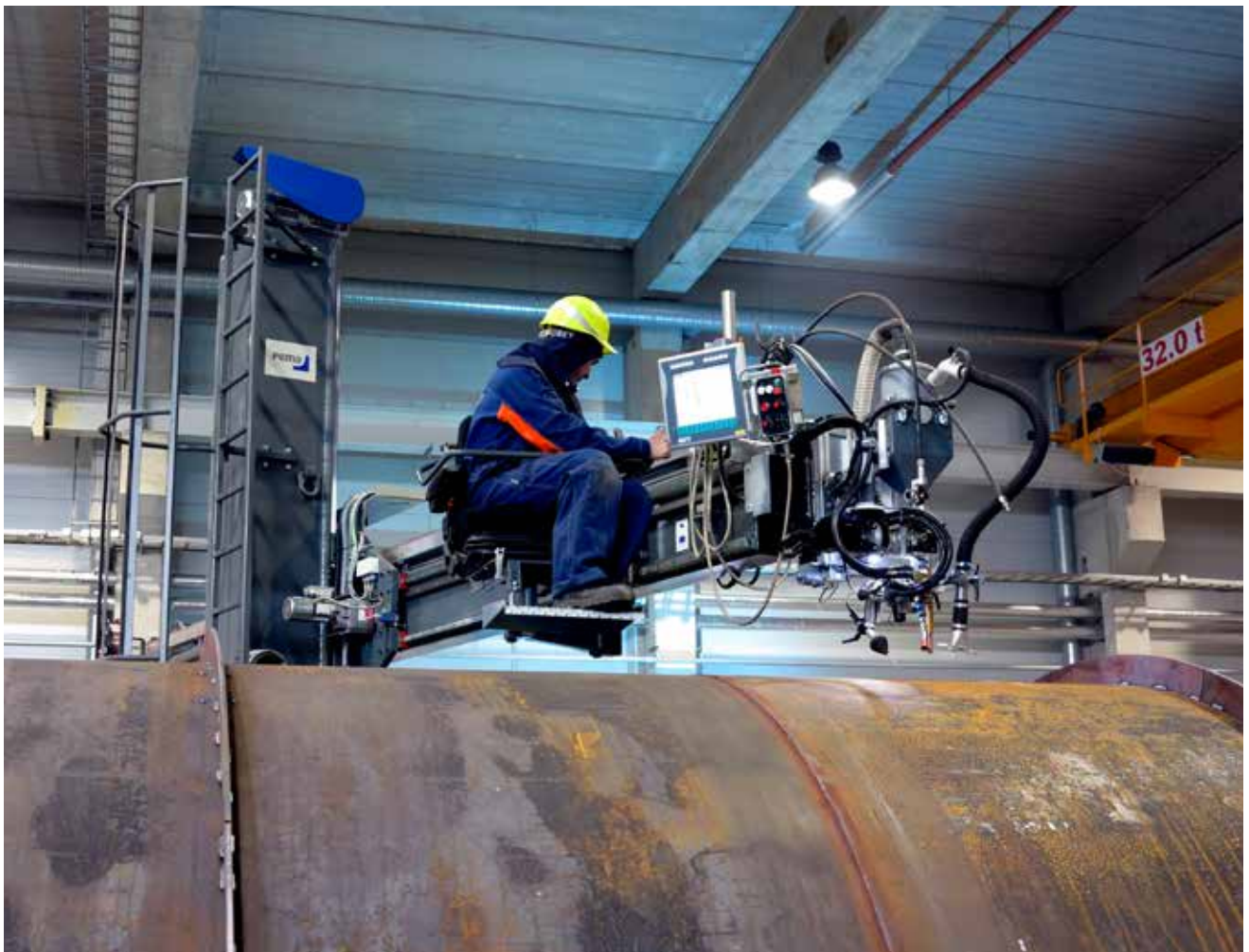
Welding with PEMA Column & Boom with PEMA WeldControl 100 system
