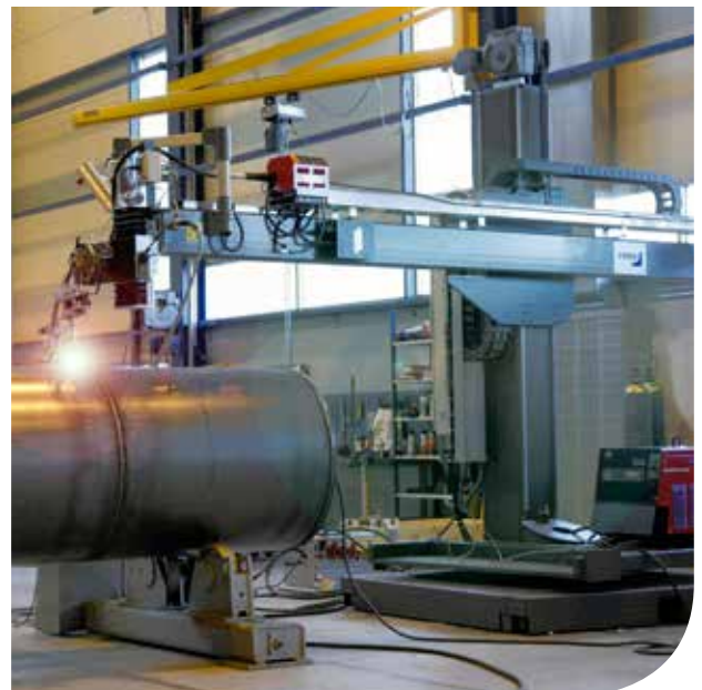
MAG welding with PEMA MD Column & Boom
