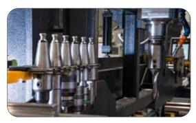
evolves from stock plates to finished plate components on one work center. The Tipo A plate processors incorporates the operations of drilling, scribing, milling, marking and tapping with thermal cutting by either oxy-fuel or plasma.
